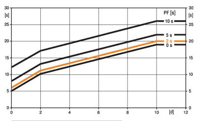
[d] = Electricity interruption in days [s] = Pre-charging time in seconds PF[s] = Bridging time Calculation example: Given an electricity interruption of 3 days and a bridging time (PF) set at 5 s, the actuator requires a precharging time of 14 s after the electricity has been reconnected (see graphic).
